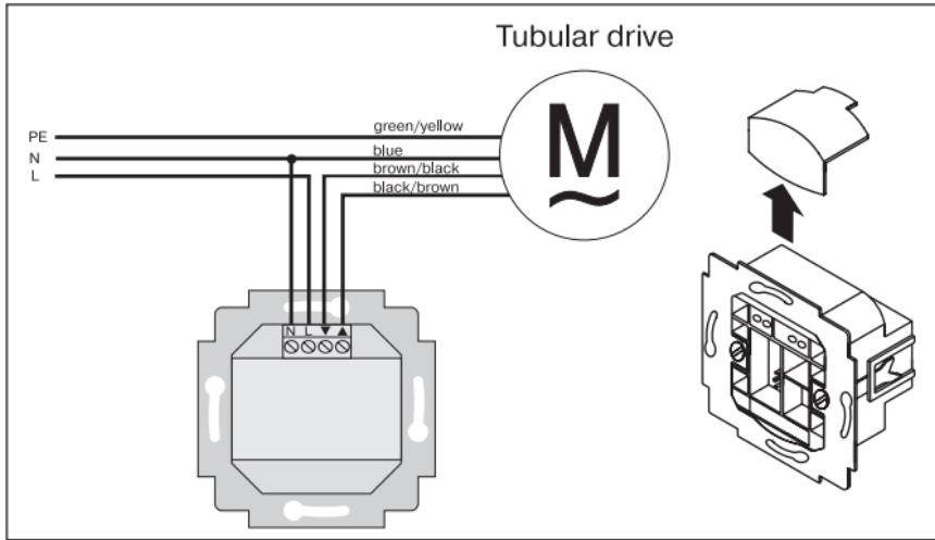
2. Put the protective cap back on the power supply unit.
